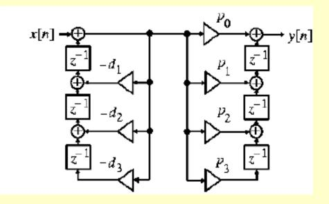
Various other noncanonic direct form structures can be derived by simple block diagram manipulations as shown below
