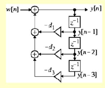
A cascade of the two structures realizing
